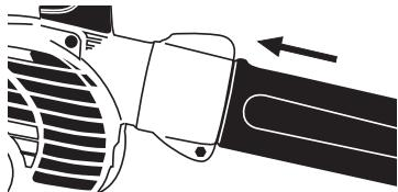
3. Rotate following the groove until you reach the locking position.. Once you have done this, you must tighten screw (a) to fix the tube.
