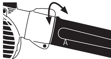
4. Open the ventilator cover by turning the knob.
