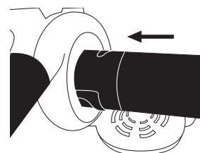
Note. This machine has a security switch that will stop the machine from working with the ventilator cover open and without the aspiration tubes being properly fitted. Check the security switch is well placed to the ventilator so that it activates once the aspiration tube has been put in place as otherwise the machine will not start.
