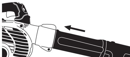
4. Rotate following the groove until you reach the locking position. Once you have done this, you must tighten screw (a) to fix the blowing tube.
